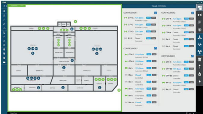
Gas tight and Blast valve monitoring and control
